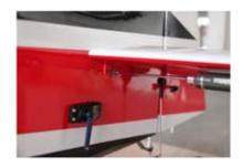
4 Connect the control horm and servo arm with ball link 50cc Interior mount
