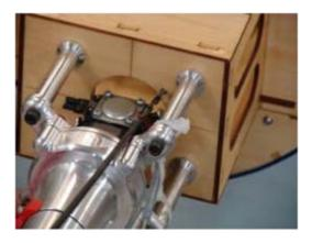
4 Attach the ball link to the throttle pushrod and secure to the carburetor throttle arm with a bolt and nylon lock nut.
