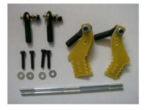
1 Connect the pushrod and control horn as shown
