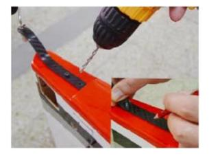
6 Insert the steering arm into the rudder steering tube and position the tube ready for gluing. Tighten the set nuts.
