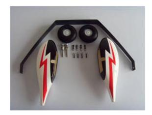
Install the landing gear in the pre-drilled holes with the supplied bolts and locking nuts.
