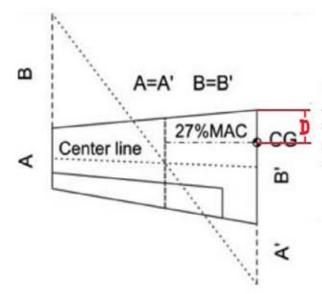
Measuer the CG from the leading edge of wing root rib. Adjust the battery pack location. For CG proper position should be at 27% MAC. This recommendation balance point is for your first flights. The CG can be moved around later to fit your personal taste.
