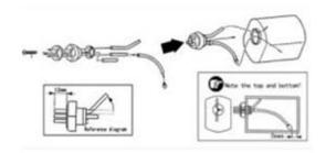
2 Assembly the outside fuel pipe as shown.
