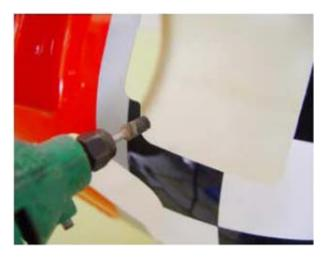
3 Use templates to cut out other opennings in the cowl for manifolds if fitted. Note: Check the engine temperature. More cut holes may be required if the engine temperature is too high.
