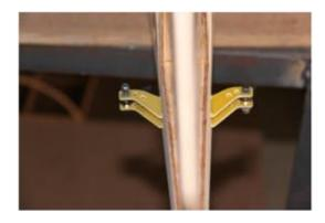
9 Use brass crimps on each cable and thread, the cable through the end of the pullpull connector.
