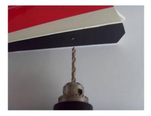
2 Assembly photo for the tail wheel parts.
