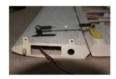
5 Repeat the previous steps for the other wing.Install the stabilizer tube and bolts.
