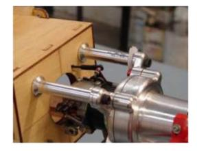
5 Insert the throttle servo into the servo mounting tray with an output arm forward.Insert the throttle pushrod into the servo arm easy link.
